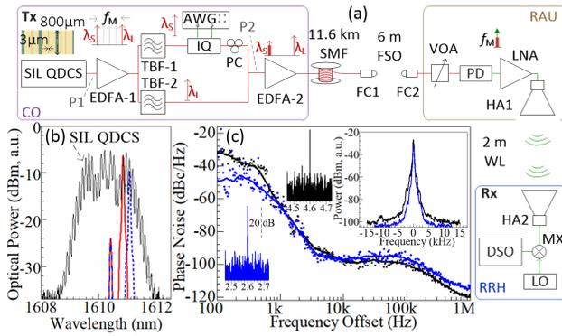
Fig. 1. (a) The experimental block diagram of the SIL QDCS source-based 50/75 GHz mmW transport system with insets depicting the schematic spectrums at selected locations. (b) Emission spectrum of SIL QDCS at location P1 and the filtered 50 (red) and 75 (blue) GHz mmW beat tones at location P2. (c) 50 (black) and 75 (blue) GHz mmW signals measured phase noise. Insets in (c) show the RF linewidths of 50 and 75 GHz mmW signals and respective coarse electrical spectrum at IFs in GHz.
