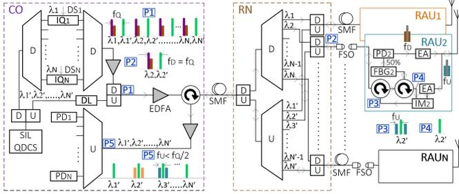
Fig. 3. Proposed RoF-RoFSO-WL hybrid network employing a single SIL QDCS with wavelength reuse feature. Inset shows the optical/electrical spectra at various locations, with half of the SIL QDCS spectrum dedicated for DS and a half for US transmission. D/U multiplexer, D/U interleaver, DL: delay line.  $f_Q$ : FSR of SIL QDCS,  $f_D$  ( $f_U$ ): DS (US) mmW carrier frequency.
