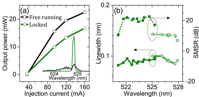
**Fig. 4.** (a) Comparison of the output optical power under the free-running and self-injection locked cases with an inset showing a free-running and locked mode at 160 mA. (b) Measured spectral linewidth and SMSR of the tunable locked modes along the tunable wavelengths at 36 mA (square symbols) and 160 mA (circle symbols) injection currents. The external cavity is fixed at 28 cm and temperature at 20°C.
