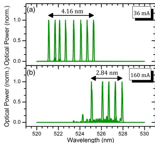
**Fig. 3.** Superimposed lasing spectra demonstrating the tunability of a green laser diode at 20°C and at (a) a low injection current of 36 mA and (b) a high injection current of 160 mA.
