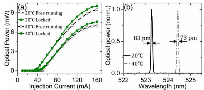
**Fig. 2.** (a) L-I characteristics of a self-injection locked tunable laser system at 20°C and 40°C. The free-running characteristics are also shown for comparison purposes. (b) Single longitudinal lasing mode operation at 36 (20) and 47 (40) mA (°C) injection currents.
