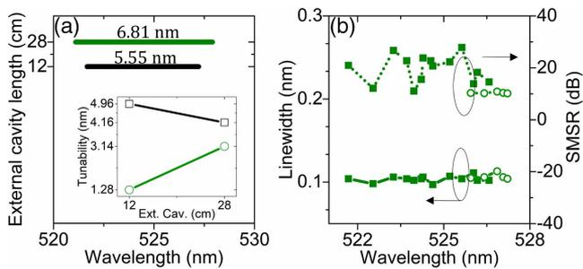
**Fig. 6.** (a) Collective tuning range of the system at low injection, 36 mA, and high injection, 160 mA, at two different external cavity lengths, and at 20°C. The inset shows the individual contributions of low (square symbols) and high (circle symbols) injection currents towards the achieved tunability. (b) Measured spectral linewidth and SMSR across the collective tuning span of 5.55 nm for low (square symbols) and high (circle symbols) injection currents at 12 cm external cavity.
