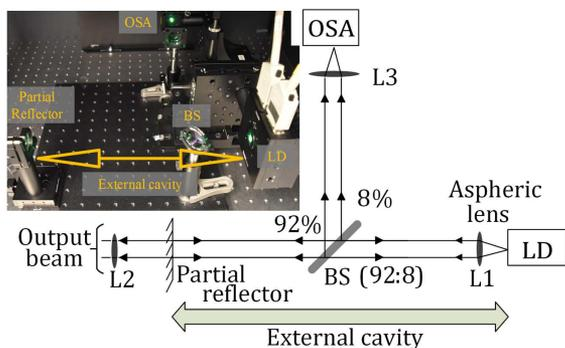
**Fig. 1.** Block diagram of a self-injection locked tunable laser system. A laboratory photograph is shown in the inset.
