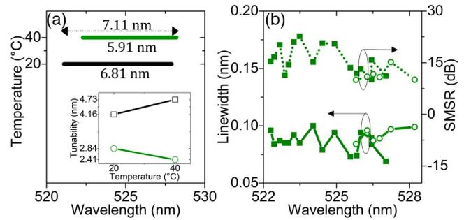
**Fig. 5.** (a) Collective tuning range of the system at low injection, 36 mA for 20°C and 47 mA for 40°C, and high injection, 160 mA at 20°C and 40°C. The inset shows the individual contribution of low (square symbols) and high (circle symbols) injection current towards the achieved tunability. (b) Measured spectral linewidth and SMSR across the collective tuning span of 5.91 nm for low (square symbols) and high (circle symbols) injection currents at 40°C. The external cavity is fixed at 28 cm.
