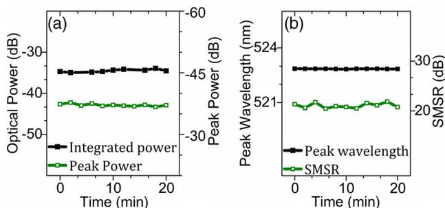
**Fig. 7.** Short-term stability of the self-injection locked tunable laser system showing the stability of (a) the total integrated and peak optical power (measured at “L3”) and (b) the peak wavelength and SMSR, of a 522.86 nm locked mode, at a 36 mA injection current, 20°C temperature, and 28 cm external cavity.
