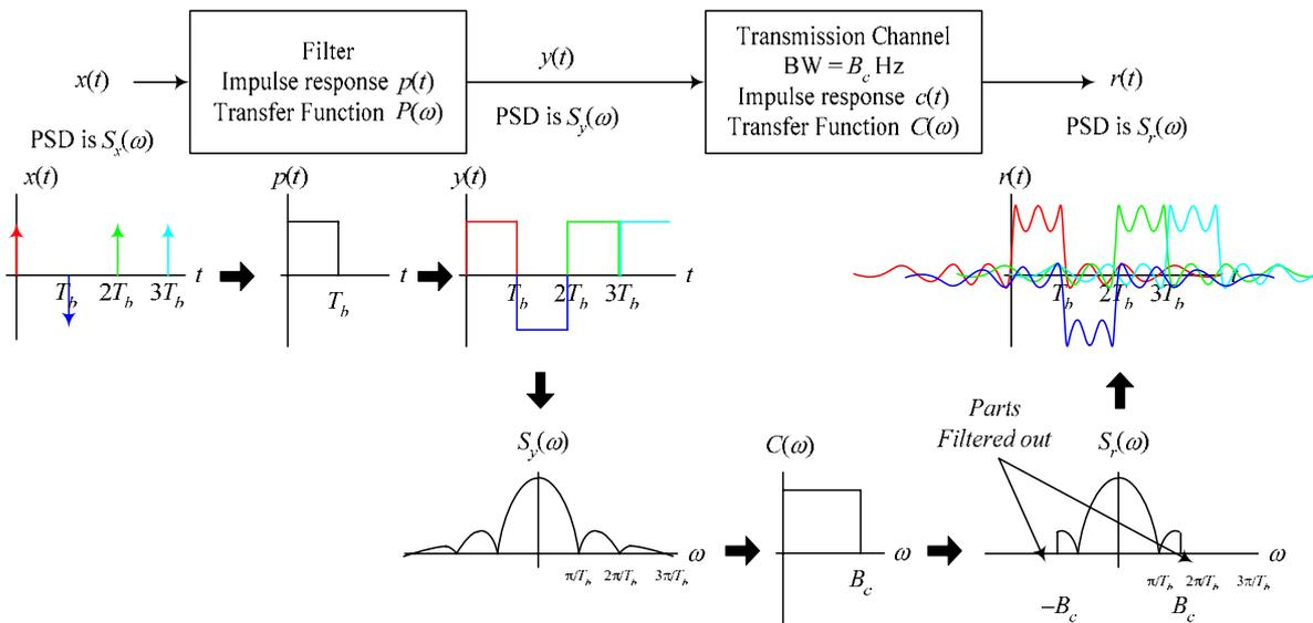
It is clear from the above figure that the square pulses in  $y(t)$  got spread out in the received signal  $r(t)$ . If the spreading is so severe, it may result in bit detection errors.
