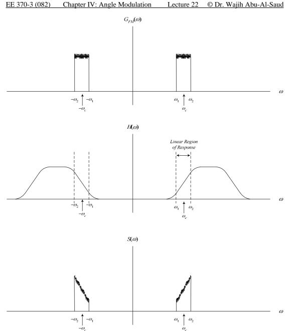
Therefore, passing the signal s(t) that is outputted by the BPF into an envelope detector gives a signal that is proportional to the message signal.
