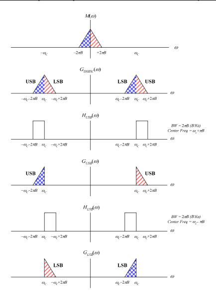
The following signal is a representation of a human voice signal. It is seen that this signal has a guard band that separates the two halves of the signal. Crating a SSB signal from this message signal is possible since a guard band of 2\*300 Hz is obtained, which means that the transition of the edge of the BPF can take place in this 600 Hz.
