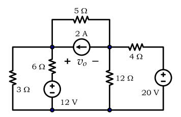
Problem 4 (25%): Use the principle of superposition to find the voltage  $V_a$  and current  $I_1$ .
