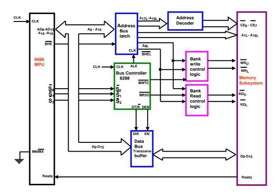
**Note:** The Bus controller is introduced here due to the support of multiprocessor environment of Maximum mode. The decoder is used to select desired memory chips. The remaining components of this circuit are similar to 8088 minimum mode circuit, as shown in <u>slide 1</u>.
