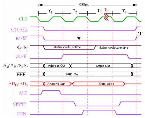
**Note:** Note that the control signal logic levels and timing diagram are similar to that of read operation, except for data transmit and receive, memory read and write signals.
