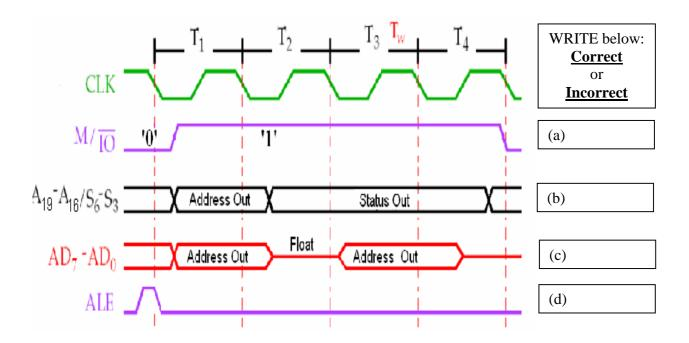
Solution: (a) Incorrect, as 8088 processors IO/M signals, and require logic '0', for the duration of the bus-cycle, to activate the memory (read) interface.
