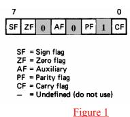
Figure 1 above shows the format of flag digits in AH register.
