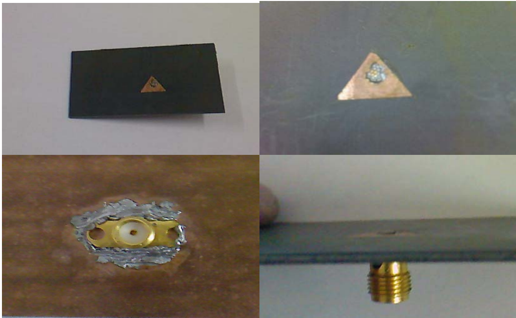
Fig.2: Upper left: the antenna. Upper right top view of the triangular patch. Lower left: bottom view of the coaxial feed. Lower right: Side view of the circuit.
