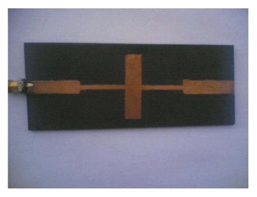
This filter is examined by the Network Analyzer and the response is the following:
