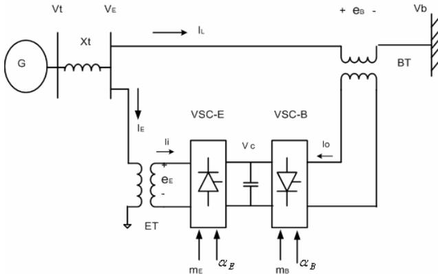
Figure 1 A single machine infinite bus system with UPFC
