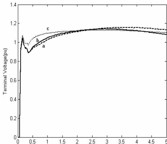
**Figure 12** Terminal voltage variation of generator following three-phase fault for different loading conditions
