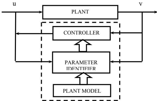
Figure 2 Block diagram of self-tuning controller
