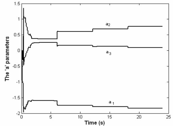
**Figure 6** Online adaptation of the 'a' parameters in the model function
