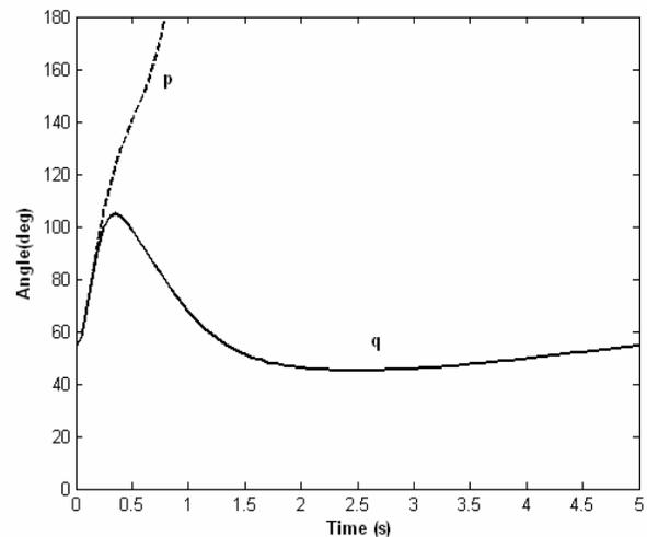
**Figure 11** Comparison of response without control (p) and the proposed adaptive control (q) following three-phase fault at 1.1 pu loading
