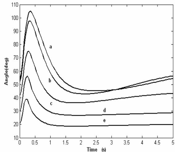
**Figure 10** Generator rotor angle following a three-phase fault for the loadings as in Fig. 9
