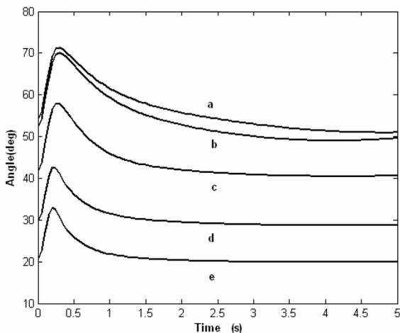
**Figure 9** Generator rotor angle variations following 50% torque pulse for 5 loading conditions.
