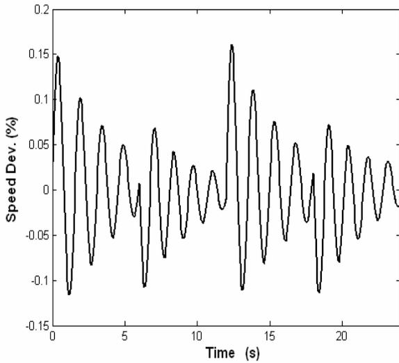
**Figure 3** Generator speed variation with no control
