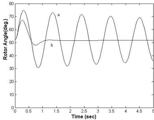
**Figure 7.** Generator rotor angle variation following a 50% input torque pulse for 0.1sec with, (a) no control, (b) proposed robust damping controller.
