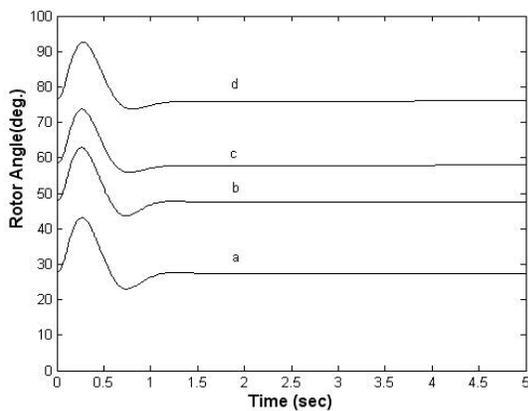
**Figure 8.** Rotor angle characteristics with the robust damping controller for (a) 0.5 pu output at 0.85 lagging pf, (b) 0.8 pu power at 0.9 pf lag, (c) 1pu power at 0.85 pf, and (d) 1.3 pu power at 0.95 pf lagging.
