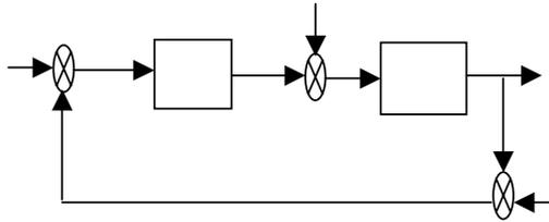
Figure 3. Unity feedback plant with controller.
