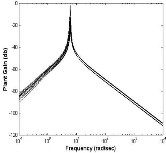
**Figure 4.** Bode magnitude diagram of nominal and perturbed plant functions
