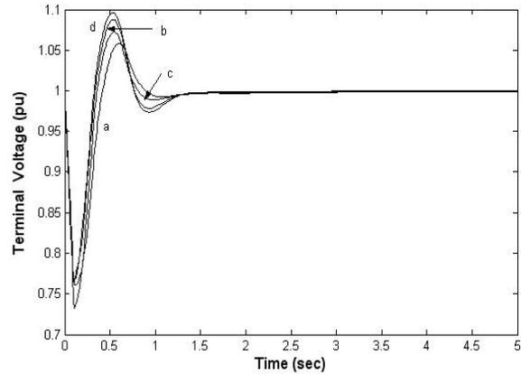
**Figure 9.** Terminal voltage variations of the generator corresponding to Fig. 8
