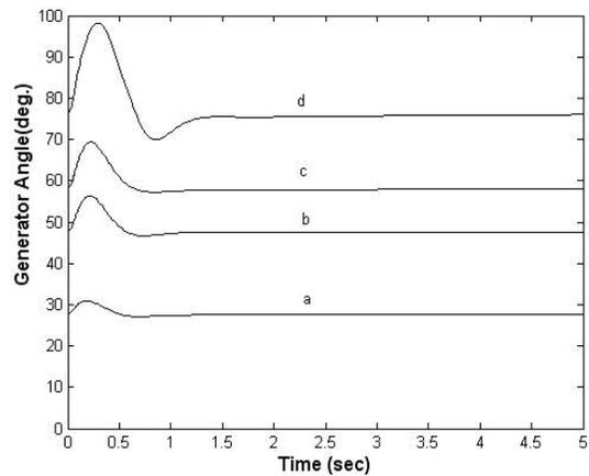
**Figure 10.** Generator rotor angle variations with the robust controller following a three-phase fault for 0.05 sec on the remote bus. The loading conditions are, a) 0.5 pu power output at 0.85 pf lag, b)0.8 pu at 0.9 pf lag, c)1pu at 0.85 pf lag and, d)1.3 pu at 0.95 lagging pf.
