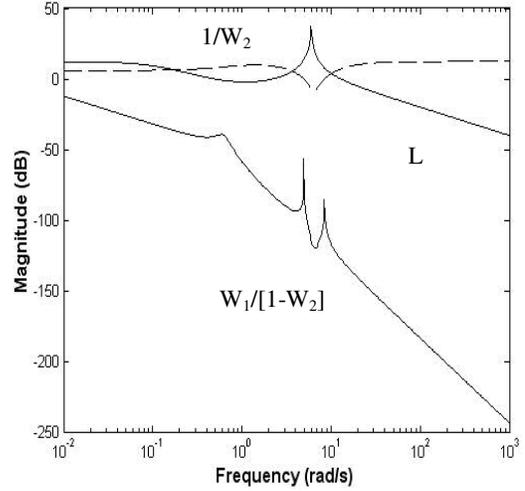
**Figure 5.** The loop-shaping boundary plots
