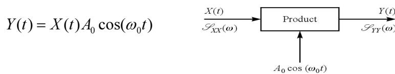
$$\begin{aligned} R_{YY}(t, t+\tau) &= E[Y(t)Y(t+\tau)] = E[A_0^2 X(t)X(t+\tau) \cos(\omega_0 t) \cos(\omega_0 t + \omega_0 \tau)] \\ &= \frac{A_0^2}{2} R_{XX}(t, t+\tau) [\cos(\omega_0 \tau) + \cos(2\omega_0 t + \omega_0 \tau)] \end{aligned}$$
