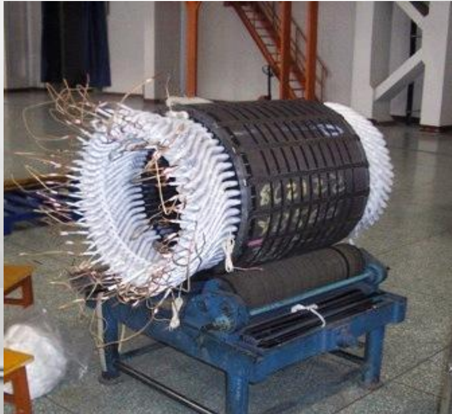
Insertion and connection of the coils
