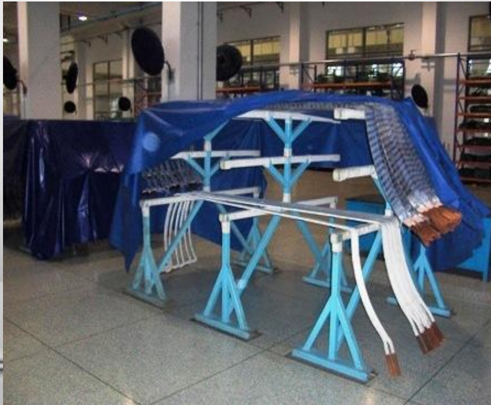
High voltage coils for 2 pole generator
