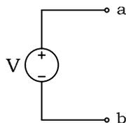
When *any* load is connected across the terminals of an *ideal* voltage source of voltage V, the same voltage V appears *across* the load, *irrespective* of the load. Note that the (+) and (-) polarities of the voltage V are on the same side.
