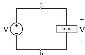
Example 1: Various *resistive* loads are connected to the 5 V ideal voltage source as shown in figure 3. In each case, the voltage across the load is also 5 V. Note that the equivalent resistance of the resistive load shown in circuit (c) and circuit (d) is considered to be the load.
