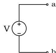
When *any* load is connected across the terminals of an *ideal* voltage source of voltage  $V$ , the same voltage  $V$  appears *across* the load, *irrespective* of the load. Note that the (+) and (-) polarities of the voltage  $V$  are on the same side.
