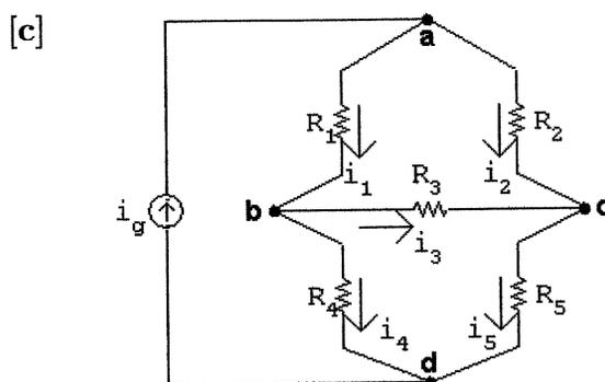
Sum the currents at any three of the four essential nodes a, b, c, and d. Using nodes a, b, and c we get
