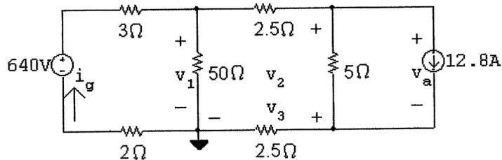
$$\frac{v_1}{50} + \frac{v_1 - 640}{5} + \frac{v_1 - v_2}{2.5} = 0 \quad \text{so} \quad 31v_1 - 20v_2 + 0v_3 = 6400$$
