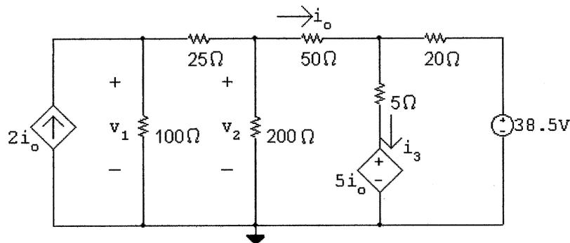
$$i_o = \frac{v_2 - v_3}{50}$$
