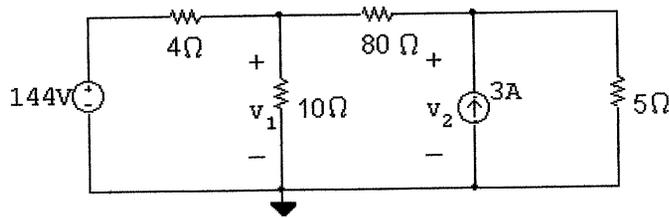
$$\frac{v_1 - 144}{4} + \frac{v_1}{10} + \frac{v_1 - v_2}{80} = 0 \quad \text{so} \quad 29v_1 - v_2 = 2880$$
