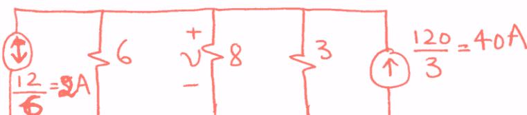
Combine two current source in parallel & 6 & 3Ω in parallel
