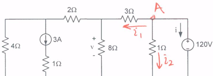
a) Resistance in series with current source & resistance in parallel with voltage source can be removed.
