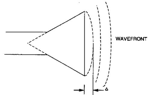
Figure (2) Phase error D of the pyramidal horn.
