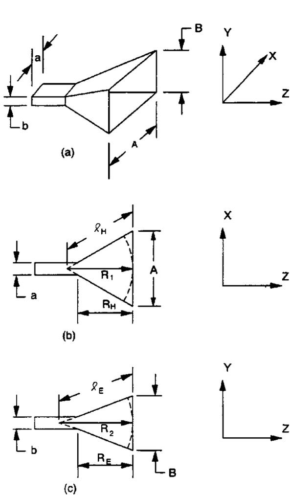
Figure (1) Geometry and dimension of the pyramidal horn.
