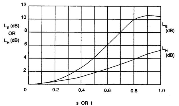
Figure (3) Loss factor for E and H plane flares.
