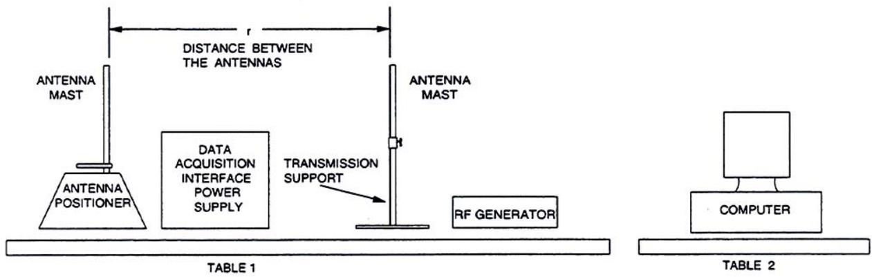
Figure 1. Set up of the ATMS modules
