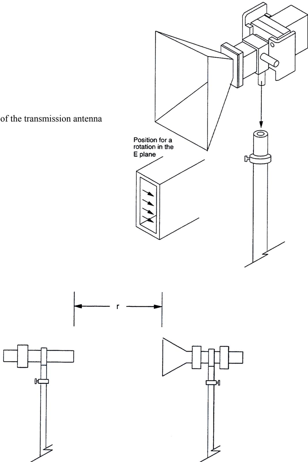
Figure 2: Distance  $r$  between the antennas
