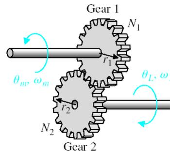
Consider the figure below, which shows a motor with inertia  $J_m$  and damping  $b_m$  driving a load consisting of inertia  $J_L$  and damping  $b_L$ . To obtain an equivalent inertia  $J$ , and equivalent damping  $b$ , we will reflect the load inertia  $J_L$  and the load damping  $b_L$  to the motor shaft.
