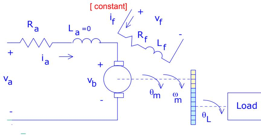
$$J_m = 5 \text{ kg-m}^2; J_L = 700 \text{ kg-m}^2; b_m = 2 \text{ N-m s/rad}; b_L = 800 \text{ N-m s/rad}; n = \frac{100}{1000}$$
