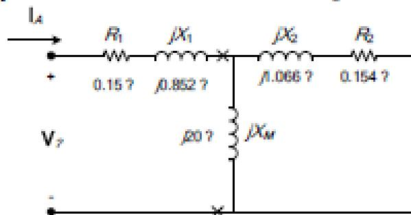
The easiest way to find the line current (or armature current) is to get the equivalent impedance  $Z_p$  of the rotor circuit in parallel with  $jX_M$ , and then calculate the current as the phase voltage divided by the sum of the series impedances, as shown below.
