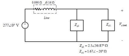
(a) The phase voltage of the equivalent Y-loads can be found by nodal analysis.
