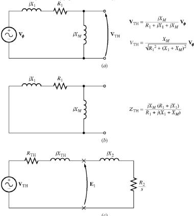
$$Z_{\mathrm{TH}} = \frac{j X_{M} \left(R_{1} + j X_{1}\right)}{R_{1} + j \left(X_{1} + X_{M}\right)} = \frac{\left(j10 \ \Omega\right) \left(0.10 \ \Omega \ + j0.21 \ \Omega\right)}{0.10 \ \Omega \ + j \left(0.21 \ \Omega + 10 \ \Omega\right)} = 0.0959 + j0.2066 \ \Omega = 0.2278 \angle 65.1^{\circ} \ \Omega = 0.0959 + j0.2066 \ \Omega = 0.2278 \angle 65.1^{\circ} \ \Omega = 0.0959 + j0.2066 \ \Omega = 0.0066 \ \Omega = 0.0066 \ \Omega = 0.0066 \ \Omega = 0.0066$$
