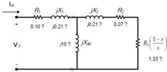
(a) The easiest way to find the line current (or armature current) is to get the equivalent impedance  $Z_F$  of the rotor circuit in parallel with  $jX_M$ , and then calculate the current as the phase voltage divided by the sum of the series impedances, as shown below.
