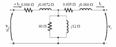
(c) To simplify the calculations, use the simplified equivalent circuit referred to the secondary side of the transformer:
