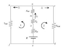
Since the magnetic device is symmetry and made by the same material at both left and right arms, we can concentrate the analysis of the circuit on either loop 1 or loop 2.
