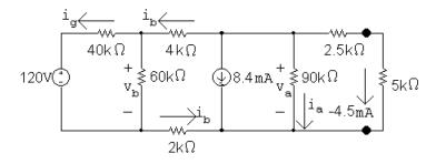
$$\begin{array}{lll} v_{\rm a} & = & (7500)(-0.0045) = -33.75 \ {\rm V} \\ i_{\rm a} & = & \frac{v_{\rm a}}{90,000} = \frac{-33.75}{90,000} = -0.375 \ {\rm mA} \\ i_{\rm b} & = & -8.4 \times 10^{-3} + 0.375 \times 10^{-3} + 4.5 \times 10^{-3} = -3.525 \ {\rm mA} \\ v_{\rm b} & = & (6000)(3.525 \times 10^{-3}) - 33.75 = -12.6 \ {\rm V} \\ i_g & = & \frac{-12.6 - 120}{40,000} = -3.315 \ {\rm mA} \\ p_{120{\rm V}} & = & (120)(-3.315 \times 10^{-3}) = -397.8 \ {\rm mW} \end{array}$$
