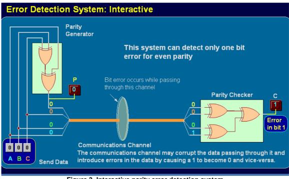
Figure 3. Interactive parity error detection system
