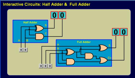
Figure 2. Interactive circuits for half adder and full adder
