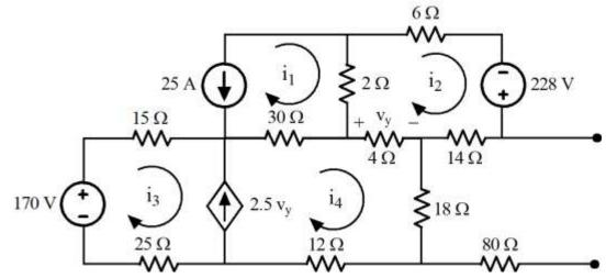
a) Find all the necessary equations to solve for the mesh currents  $i_1$ ,  $i_2$ ,  $i_3$ , and  $i_4$ . [Note: In this part do not simplify or solve any system of equations]
