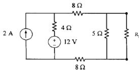
For the circuit shown above find the maximum power absorb by the load resistor R<sub>L</sub> ?
