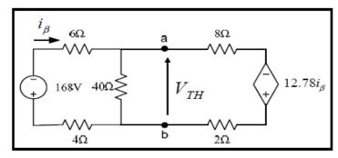
Then, we calculate the short-circuit current  $I_{sc}$  using the circuit below:
