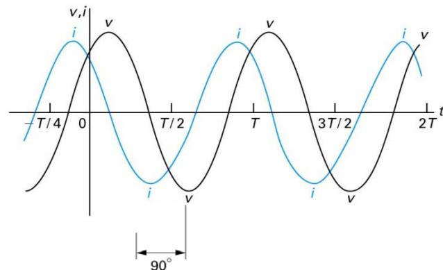
→ The sinusoidal voltage and current in an **inductor** are **out of phase** by  **$90^\circ$**
