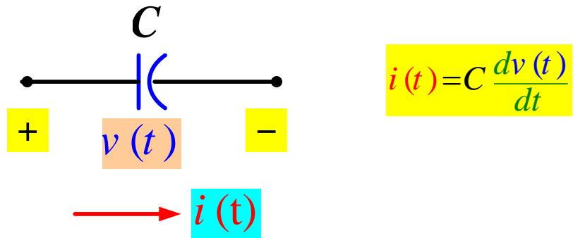
Let the voltage across the capacitor be a **sinusoidal** given as  $v(t) = V_m \cos(\omega t + \theta_v)$
