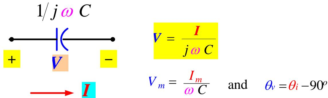
The voltage **lag** the current by **90°** or the current **lead** the voltage by **90°**
