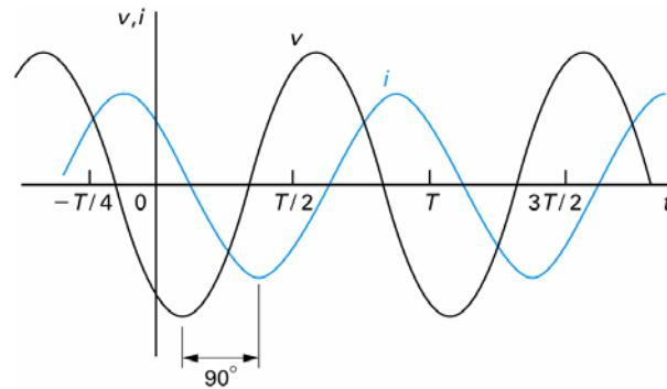
→ The sinusoidal voltage and current in an **inductor** are **out of phase** by **90°**
