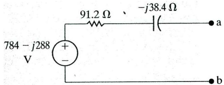
$$Z_{Th} = \frac{V_T}{I_T} \quad \text{Find } I_T \text{ in terms of } V_T \text{ then form the ratio } \frac{V_T}{I_T}$$
