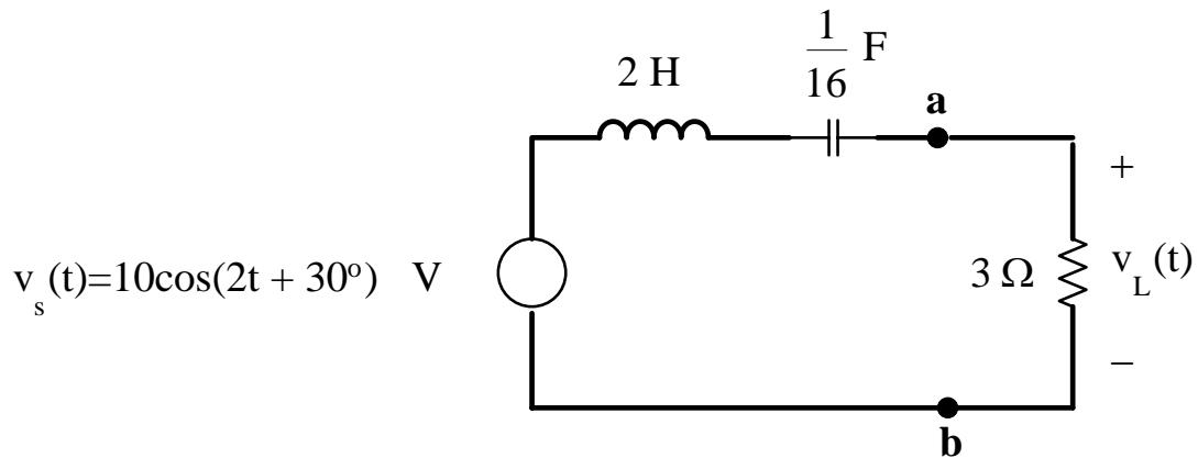
Using the Thevenin Reduction Method only, find  $V_L(t)$  the voltage across the load resistor  $3 \Omega$  ?
