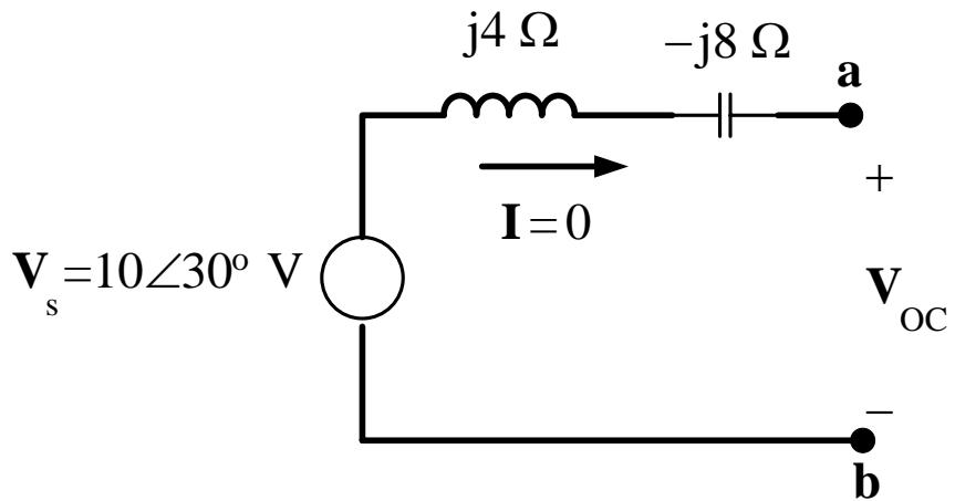
$$\Rightarrow V_{OC} = V_s = 10\angle 30^\circ \text{ V}$$
