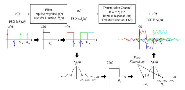
It is clear from the above figure that the square pulses in y(t) got spread out in the received signal r(t). If the spreading is so severe, it may result in bit detection errors.
