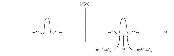
Adding the spectrum of the different signals like z(t) given above will give us the spectrum of the approximation signal  $\hat{g}_{FM}(t)$
