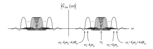
If we assume that the sidebands (the small humps at the two edges of a sinc function) have negligible power, and knowing that  $\Delta \omega = k_f \cdot m_p$ , we see that the bandwidth of an FM signal is approximately equal to
