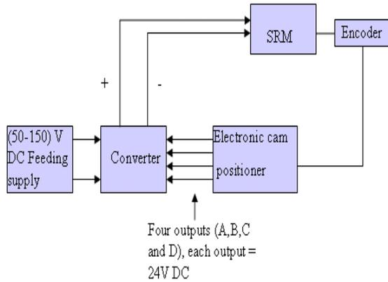
Fig. 4: The Block Diagram for the Control System of SRM.
