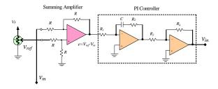
Fig. 4 Analog implementation of the PI controller
