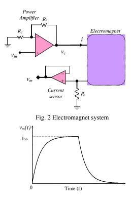
Fig. 3 Step response of the electromagnet
