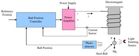
Fig. 1 Magnetic levitation system
