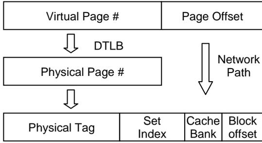
Figure 4: Network path establishment can be done in parallel with DTLB virtual address translation
