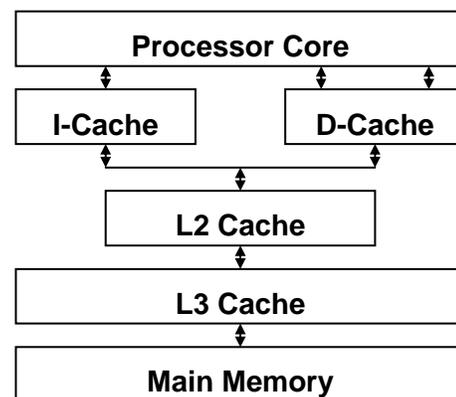
Figure 1: Cache hierarchy for a typical wide-issue superscalar or a small scale SMT architecture
