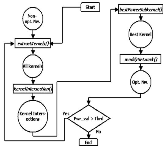
Figure 1. A flowchart for the overall optimization process targeting low power
