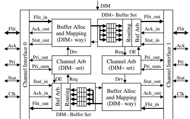
Figure 5: Internal Structure of a Router
