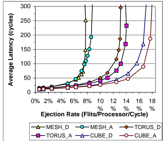
Figure 10: Average latency and Ejection Rate in a 3D Mesh, a 3D Torus, and a 9D Hypercube
