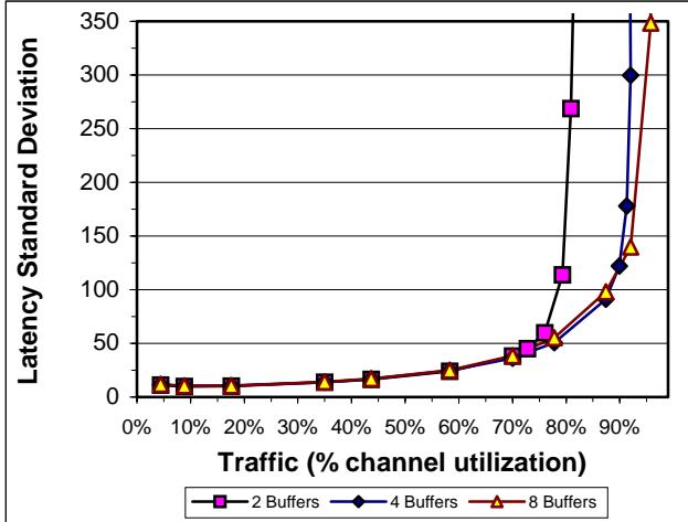
Figure 9: Latency Standard Deviation and Traffic in an 8x8x8 Torus
