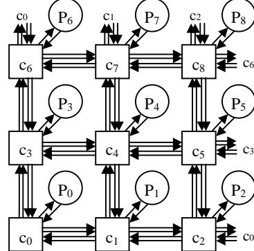
Figure 4: Graph model of a 3-ary 5-way torus
