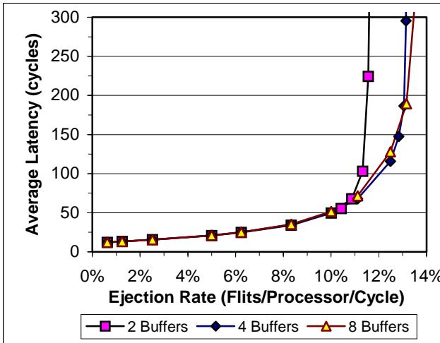
Figure 8: Average latency and Ejection Rate in an 8x8x8 Torus
