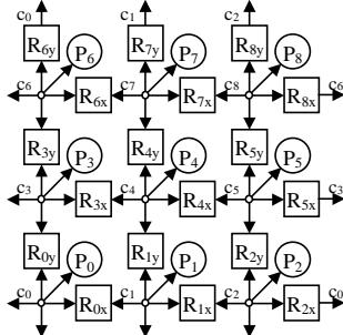
Figure 1: A 3-ary 5-way torus processors linked to channels
