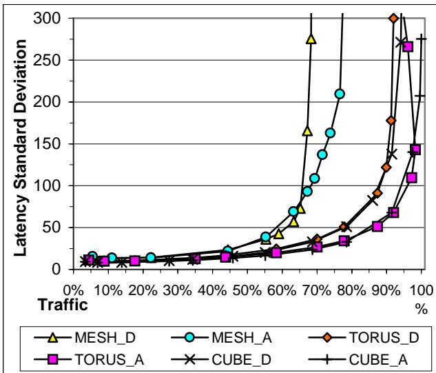
Figure 11: Latency Standard Deviation and Traffic in a 3D Mesh, a 3D Torus, and a 9D Hypercube
