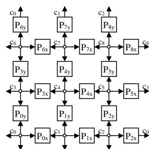
Figure 2: A 3-ary 4-way torus processors linked to routers
