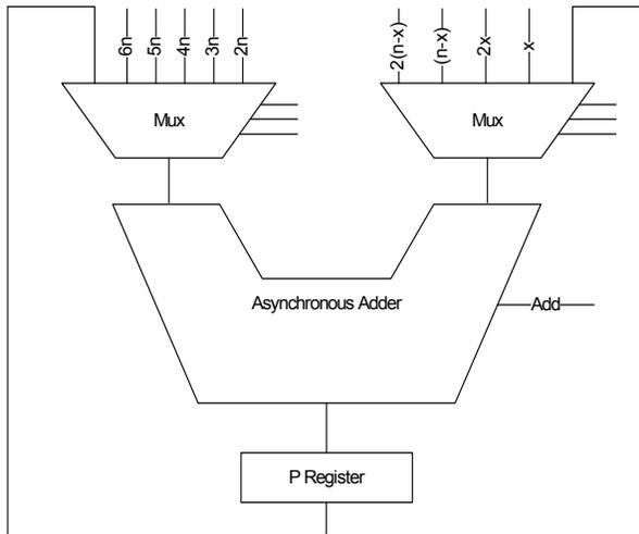
**Figure 3:** Asynchronous Multiplier Data Path.
