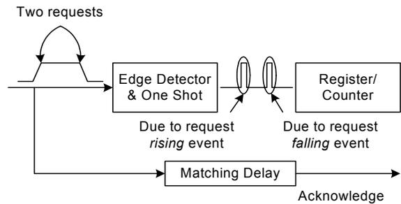
**Figure 5:** Clock Pulse Generation for GALS Designs.
