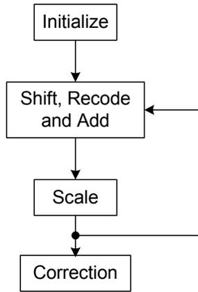
**Figure 2.** Data flow of the Modular Multiplication Algorithm
