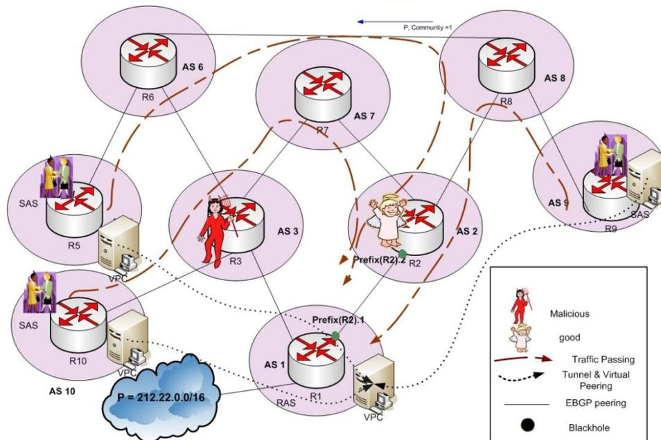
**Figure 17: Virtual peering-based solution.**
