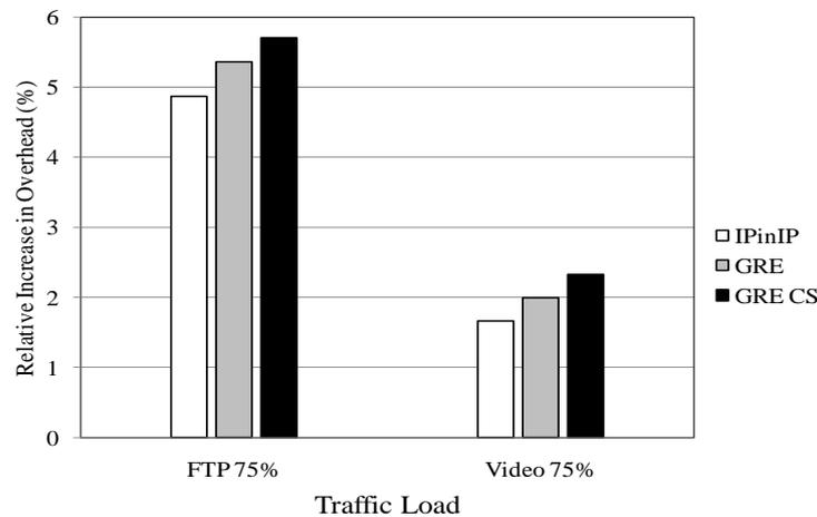
**Figure 24: Relative increase in throughput overhead.**
