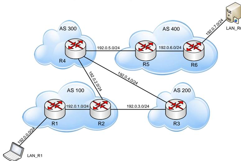
**Figure 2: The lab testbed resembling a typical network configuration.**
