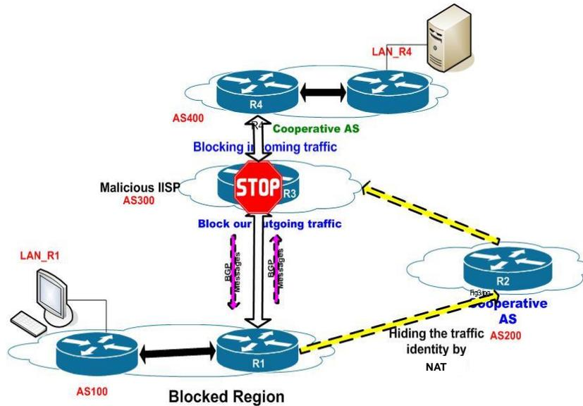
**Figure 33: NAT-based solution laboratory testbed setup**
