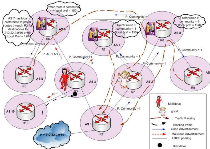
Figure 12: Control the traffic through the use of communities.
