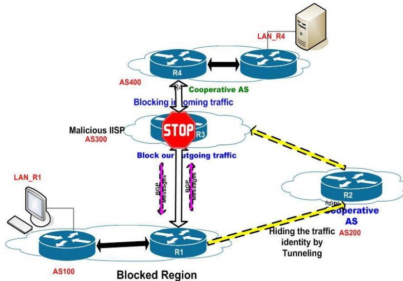
**Figure 26: Tunnel-based solution laboratory testbed setup**
