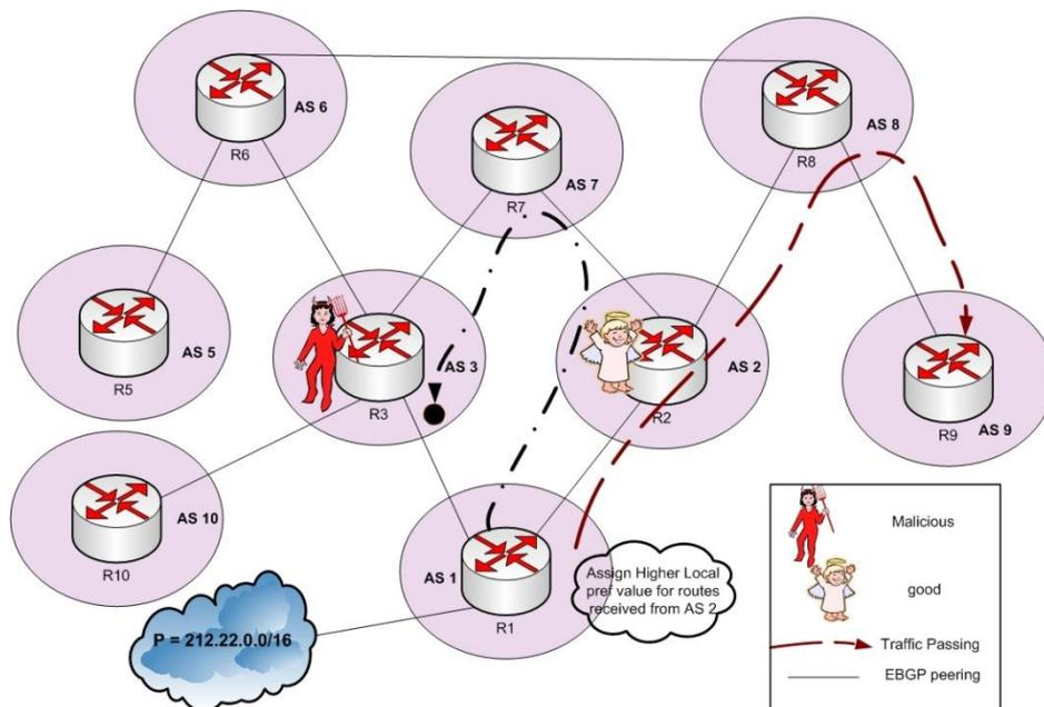
**Figure 9: Control of outgoing traffic using BGP tuning.**
