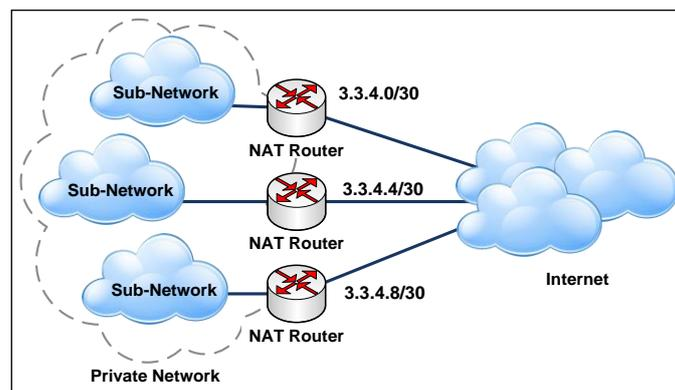
**Figure 27: Extended NAT design using load-balancing over a number of NAT routers.**
