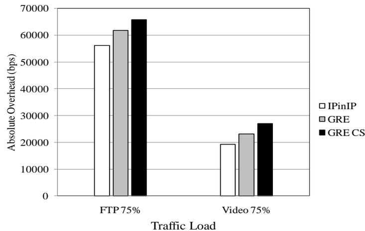
**Figure 25: Absolute throughput overhead.**
