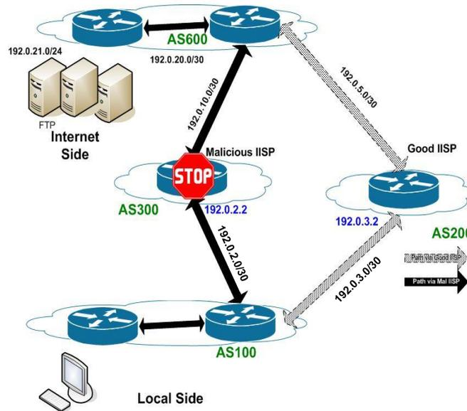
**Figure 15: BGP-based solution laboratory testbed setup**
