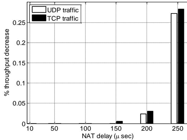
**Figure 32: Relative decrease of throughput for high TCP and UDP traffic.**
