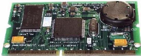
Figure 4. Tini microcontroller
