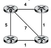
Suppose that the link cost c(0,1) has changed from 4 to 1, re-compute the distance tables for nodes 0, 1, 2, and 3 after each iteration of a synchronous version of the distance vector algorithm using as many of the following tables as needed. Note that the current tables' values <u>prior</u> to the link cost change are as shown in the leftmost column of the tables.
