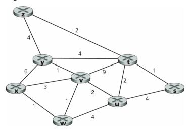
With the indicated link costs, use *Dijkstra*'s shortest-path algorithm, <u>as discussed in class</u>, to compute the shortest path from y to all network nodes using the table given below.
