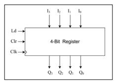
Design the counter using this register together with a 4-bit binary parallel adder, a single OR gate and any other MSI parts.
