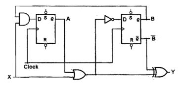
b. Give logical expressions for the D inputs of the flip flop and for the external output
