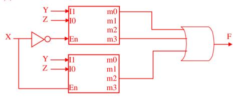
**b.** Implement F using the 4-to-1 MUX shown below (see steps for obtaining the solution)
