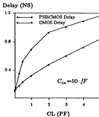
Fig.4. Delay vs load capacitance of the CMOS buffer chain and the PSBiCMOS buffer.
