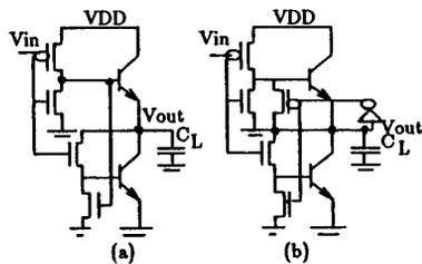
Fig.1. (a) A partial swing BiCMOS (PSBiCMOS) Buffer, (b) A full swing BiCMOS (FSBiCMOS) buffer.
