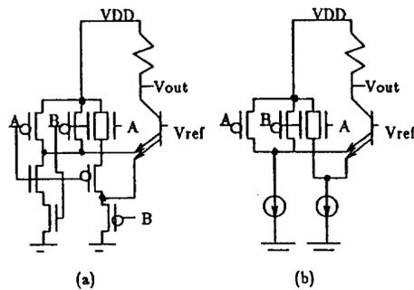
Fig. 9. XOR implementation using: (a) a LPM<sup>3</sup>BiCML, and (b) a M<sup>3</sup>BiCML structures.
