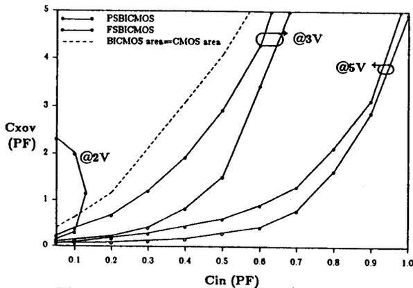
Fig.5. The cross-over capacitances vs Cin for the three BiCMOS technologies.
