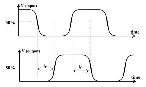
Average propagation delay  $T_D = (t_r + t_f)/2$
