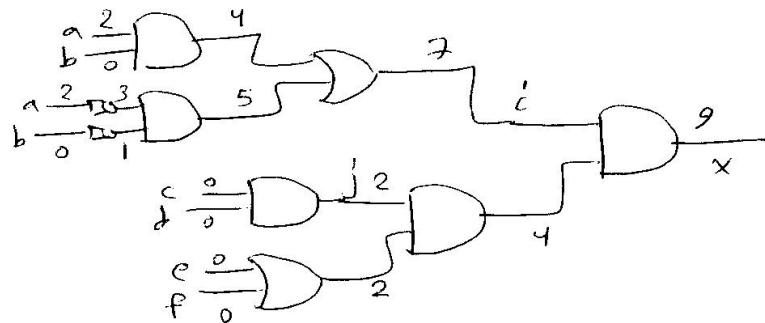
This, delay of x is reduced from 12 to 9. At the same time, the area of the circuit has improved.
