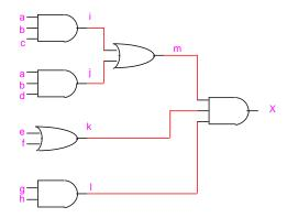
Assume that the delay of a gate is related to the number of its inputs i.e. the delay of a 2-input AND gate is 2. Also, assume that the input data-ready times are zero for all inputs.
