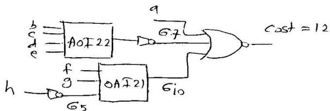
This solution is obtained by adding a cascade of inverters at the output of G7.
