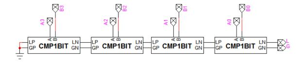
The model for a 1-bit comparator is as follows:
