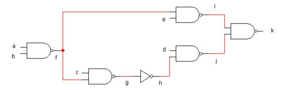
Assume that the delay of the inverter gate is 1 and that the delay of the 2-input NAND gate is 2. Also, assume that the input data-ready times are zero except for input *a*, which is equal to 2.
